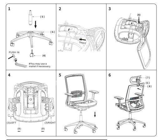
Insert and loosely tighten all screws. When assembly is completed, fully tighten all screws before using. This chair is only intended for sitting. Any other use will void the warranty.
