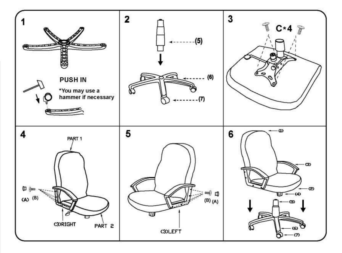
It is important to assemble all parts so that the directional "Arrows" point in the same direction. Make certain that all screws are FULLY tightened before using the chair. Each month, check all screws and tighten any that may have loosened.
