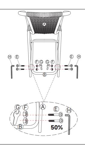
STEP 3 Completely tighten all screws.
