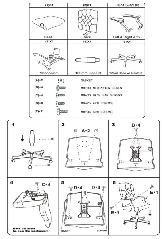
Insert and loosely tighten all screws. When assembly is completed, fully tighten all screws before using. This chair is only intended for sitting. Any other use will void the warranty.
