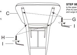
STEP 5B: Attach Seat Back (Part C) to the upper part of the Metal Tube Frame (Part A) using M6\*35 Screws (Part G) and Large Allen Wrench (Part I)
