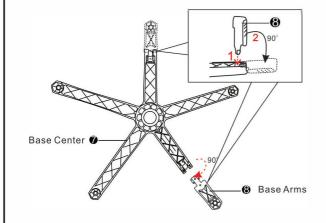
STEP 2: Insert (5)Casters (Part 9) into the base arms and return base assembled base to the upright position. insert the wide end of the Gas Lift (Part 6) into the Base Center. Slide the Gas lift Cover (Part 5) downwards over the Gas Lift .
