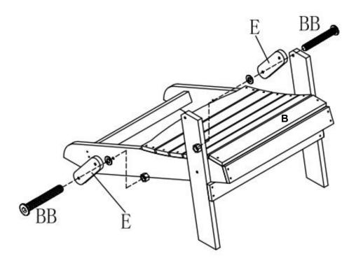
Attach the right armrest (Part C) and left armrest (Part D) to the legs (Part F) with M8\*50 bolts bolts (Part BB)
