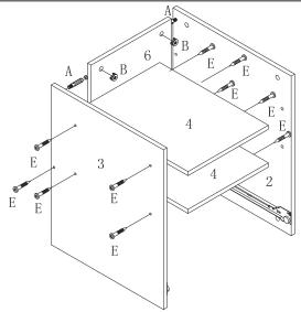
Attach left side panel (Part 3) and right side panel (Part 2) to upper and lower shelves (Part 4) using 8 screws (Part E). Attach back panel (Part 6) to left and right side panels using joint connector nut (Part B) and dowels (Part A). Insert 2 remaining screws (Part E) on left and right side panels and tighten.
