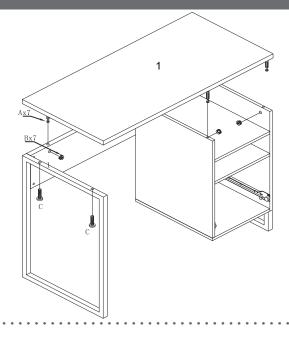
Attach desktop (Part 1) to frame using joint connector nuts (Part B) and dowels (Part A). Insert bolts (Part C) through the underside of left metal frame and tighten.
