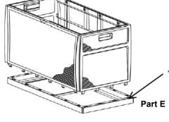
Tip: Put the flat border face with holes upwards.
