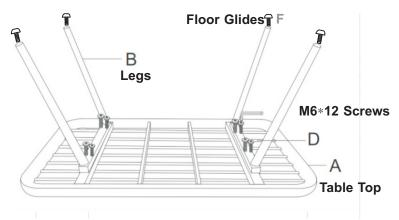
STEP 1: Attach (2) Legs (Part B) to the underside of Table Top (Part A) using (8) M6\*12 Screws (Part D). Tighten using Allen Wrench (Part E). Insert Adjustable Glides (Part F) and turn to desired height to level the table.
