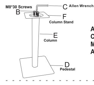
Attach the Column (Part E) to the Column Stand (Part F) using (3) M8\*30 Screws (Part B). Tighten using Allen Wrench (Part C).
