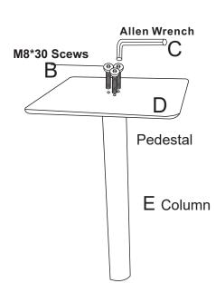
Attach the Pedestal (Part D) to the Column (Part E) using (3) M8\*30 Screws (Part B). Tighten using Allen Wrench (Part C).
