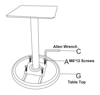
Lay Table Top (Part G) upside down on a smooth clean surface and attach the assembled column using (4) M6\*12 Screws (Part A). Tighten using Allen Wrench (Part C).
