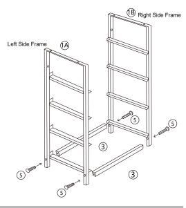
STEP 1: Attach Left Frame (Part 1A) and Right Side Frame (Part 1B) to the Frame Poles (Part 3) using (4) M6x25mm Screws (Part 5)
