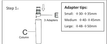
Insert the correct adapter (Part E) for your umbrella into the Column (Part C).
