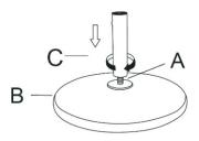
Turn the Column (Part C) clockwise to tighten.
