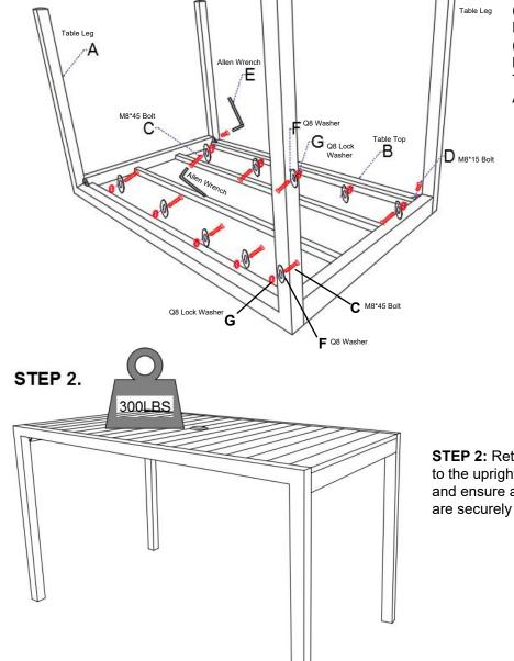
STEP 1B: Secure corners of Table Top (Part B) to Left and Right Table Legs (Part A) using (4) M8\*15 Bolts (Part D). Tighten all bolts using Allen Wrench (Part E)
