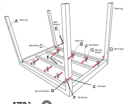
STEP 1B: Secure corners of Table Top (Part B) to Left and Right Table Legs (Part A) using (4) M8\*15 Bolts (Part D). Tighten all bolts using Allen Wrench (Part E)
