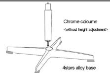
Place the column onto the base
