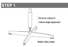
Place the column onto the base
