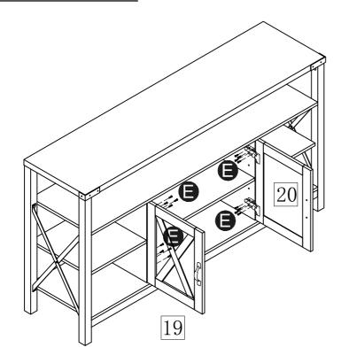
Attach the other end of the hinges to the inside of the Center Panels using (16) 3.5\*14MM Screws (Part E). Tighten or loosen the screws to ensure a proper fit.
